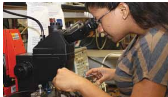
Capacitance - Voltage measurements in progress to study the dielectric/GaN interface
